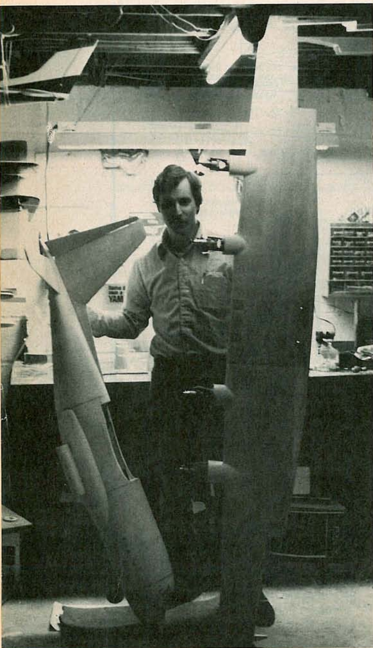
The realistic appearance of the Hercules has been achieved without a lot of intricate detailing. This is a scale project intended to be practical for use as a sport model. Here we see the plug for the fiberglass cowlings and several finished units (top). The construction method used for the fuselage permits compound curves to be duplicated with relative ease (left). This is a big model with a 7\frac{1}{2} foot span.
