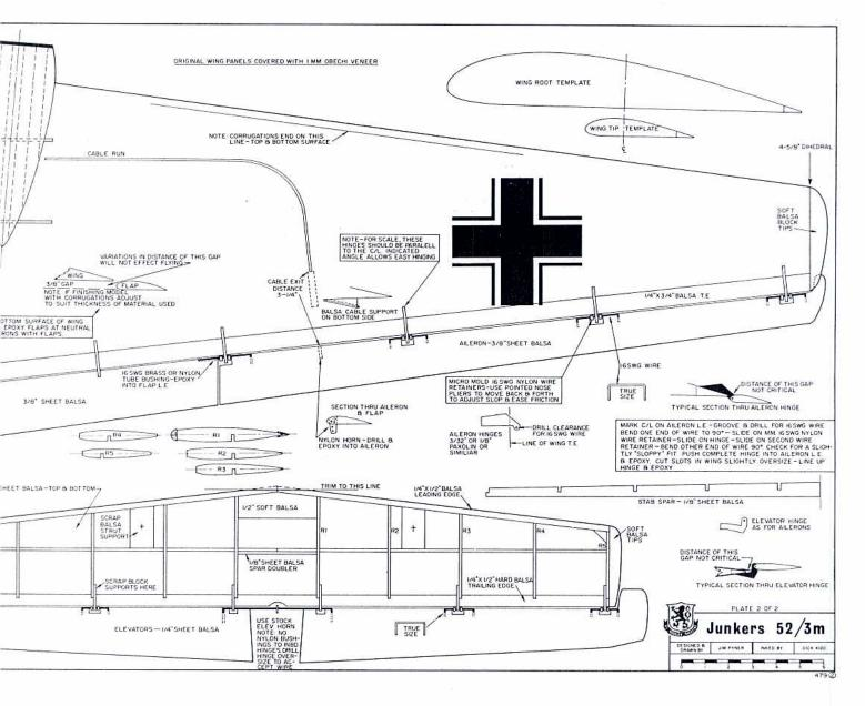
particular here. Just standard multi practice. The elevators are cut from 1/4" firm sheet, joined with a stock elevator rod and horn. Study the hinge detail on the plan. Cut the hinges from paxolin or similar plastic and drill for 16 SWG wire. Drill two oversize to accept the thicker wire of the elevator joiner. Mark a centre line on the L.E. of the elevator, drill and groove for the hinges.
