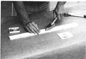
Iron X-hinge down on elevon (both sides).
