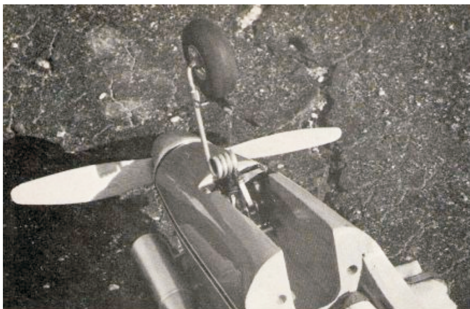
Close-up of the ProLine nose wheel installation. ProLine retract gear is a Chidgey design.
